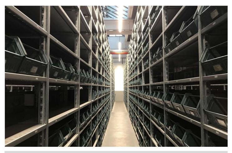
The shelves had to be rearranged in the tool store. This led to insufficient lighting. The conventional lighting did not take into account the uniform illumination of the vertical surfaces, the storage media and their contents.
