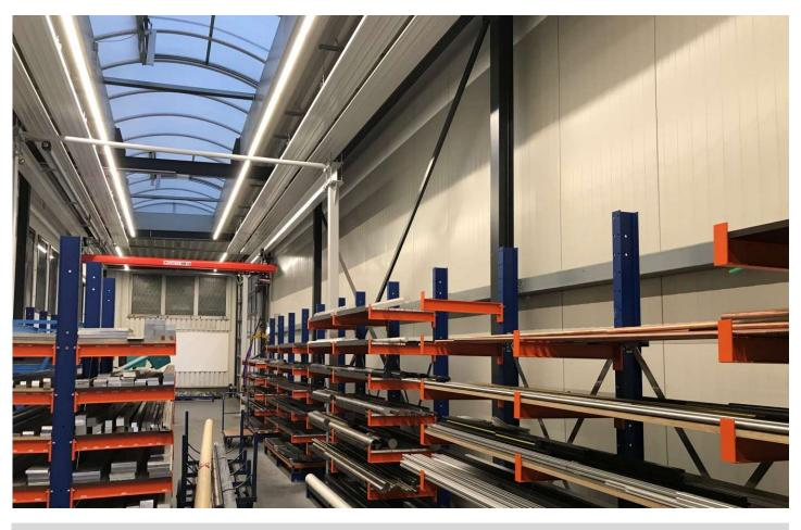
The bar storage system was rebuilt and was no longer adequately lit due to the new arrangement of shelves and storage areas. The existing lighting did not take into account the illumination of the vertical storage areas.
