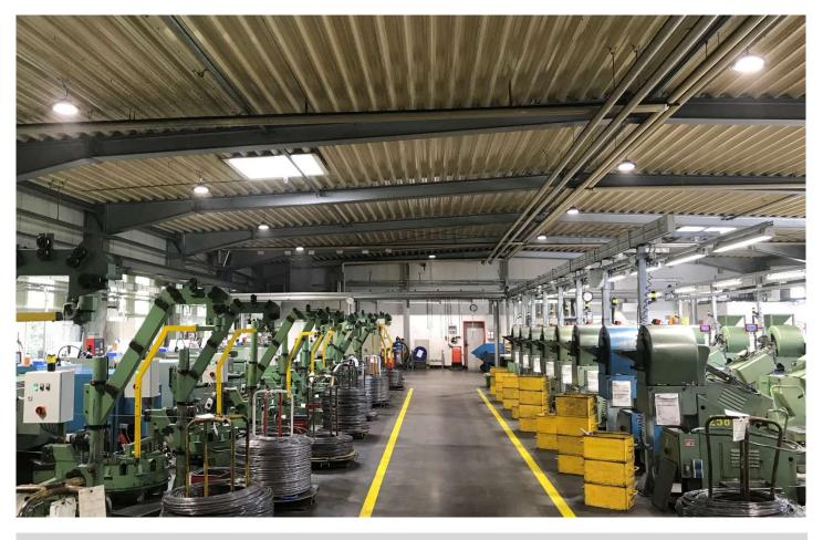
In the pressing plant with wire storage next to it, cold formed parts are produced in 3-shift operation. The pressers have different tasks and visual performances on the machines. The existing illumination had become inadequate due to the use of space, the daylight incident, the positioning of the machines and the changes in visual tasks.
