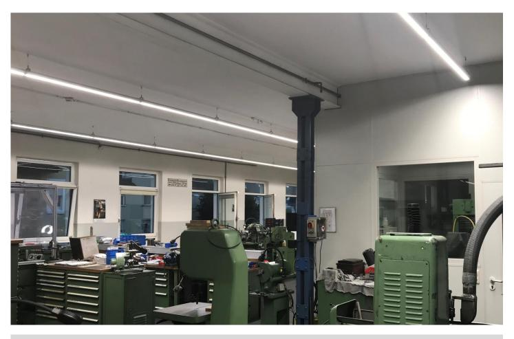
The tool making department including the adjoining rooms (locksmith's shop and hardening shop) was not sufficiently illuminated. 1xT8 58W and 2xT8 58W continuous row luminaires no longer met the lighting requirements for workplace lighting. The average illuminance in the working plane level was less than 500 lux. The maintenance costs were negatively affected by frequent lamp changes. The energy costs were too high.
