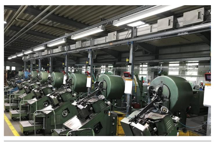
For the "Metal working" department and its 2-shift operation, the illumination should become more efficient and brilliant. The visual conditions at the machines were inadequate. The illuminance in the working plane level was below the recommended values. In use were 21x 1xT5 54W classic fluorescent lamps with high energy consumption. The maintenance costs were negatively affected by frequent lamp changes.
